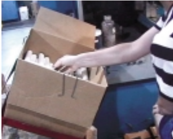
A tilted box with clips reduces wrist bending.
