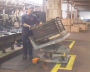
A lift and tilt table reduces bending by providing easy access to parts.
