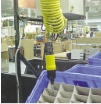
A powered hand tool that is balanced, properly oriented and has good handle design.
